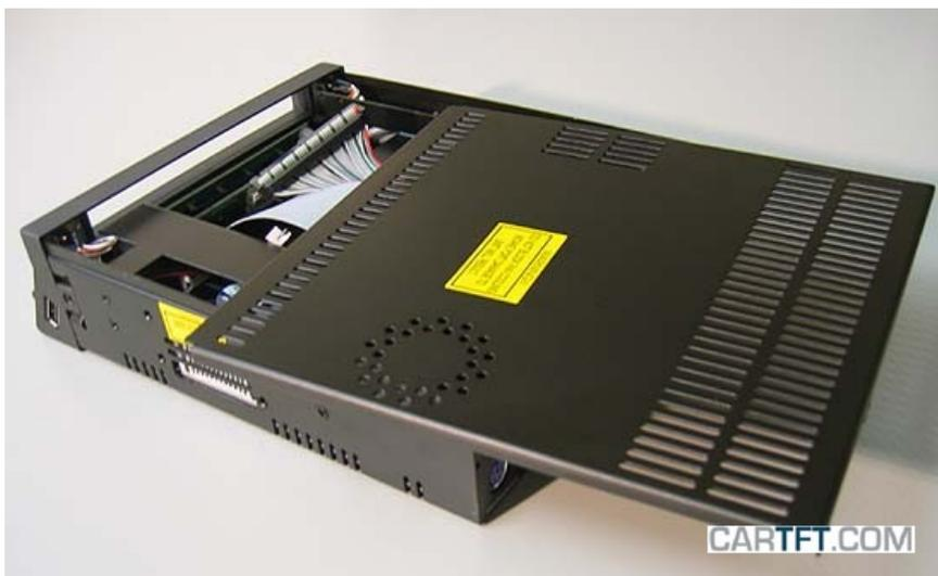
Remove each 4 screws, on the left and on the right side of the casing, which hold the inner framework.
