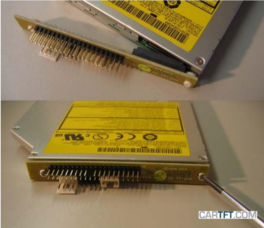
Sliding now the Slimline disk drive of the front into the track by the case disk drive slit until the screw holes of the Slimline disk drive lie at the 2 corresponding openings → then screw them tight.
